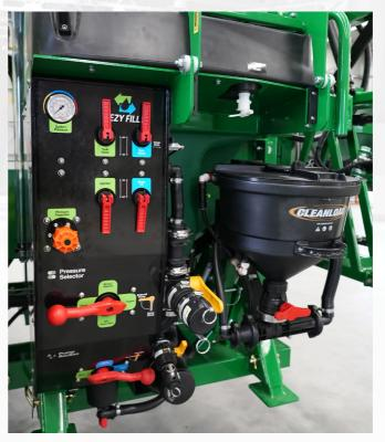
Sprayer controls are clearly labelled, flip valves control all suction, pressure and filling functions.
